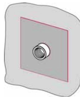
Fig. 2: Bedding the sealing sleeve into the still-wet sealing coating
