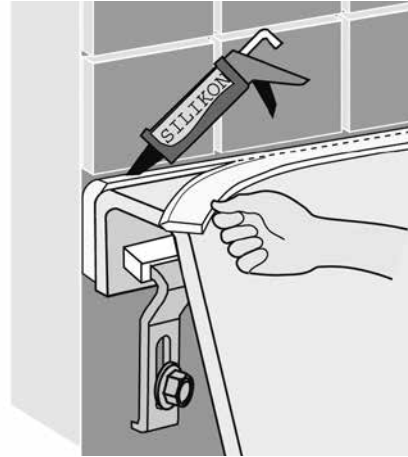
Sealing with bathtub insulation tape and a silicone joint
