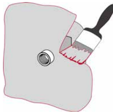
Fig. 3: Applying the upper sealing coating
