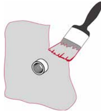
Fig. 1: Applying the lower sealing coating
